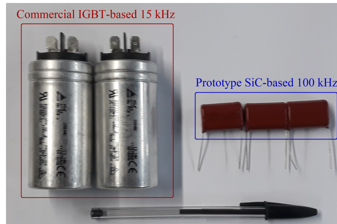
Figure 12. Size comparison between filter capacitors for the developed SiC-based prototype and for a commercial IGBT-based UPS with the same specifications.
