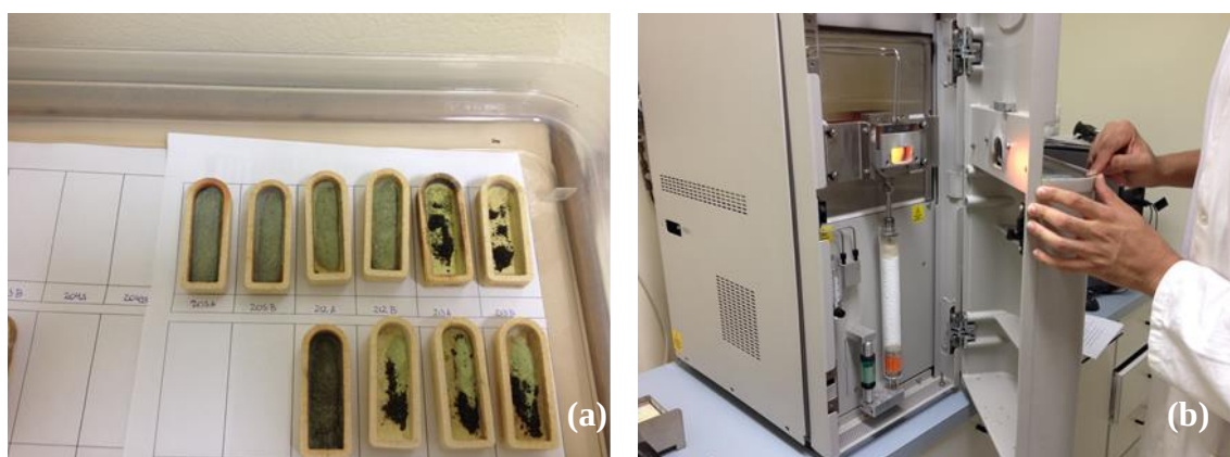
Figure 2.13: (a) Aggregate sample for direct combustion test (b) Equipment LECO SC 632 (MARCELINO, 2015).
