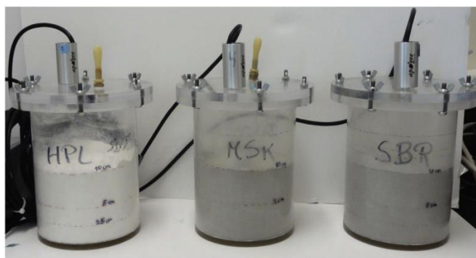
Figure 2.22: Oxygen consumption test (RODRIGUES et al. , 2016a).
