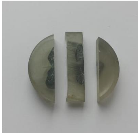
Figure 4.31: Block sawn of sample 4.80 oxidized for MLA analysis.
