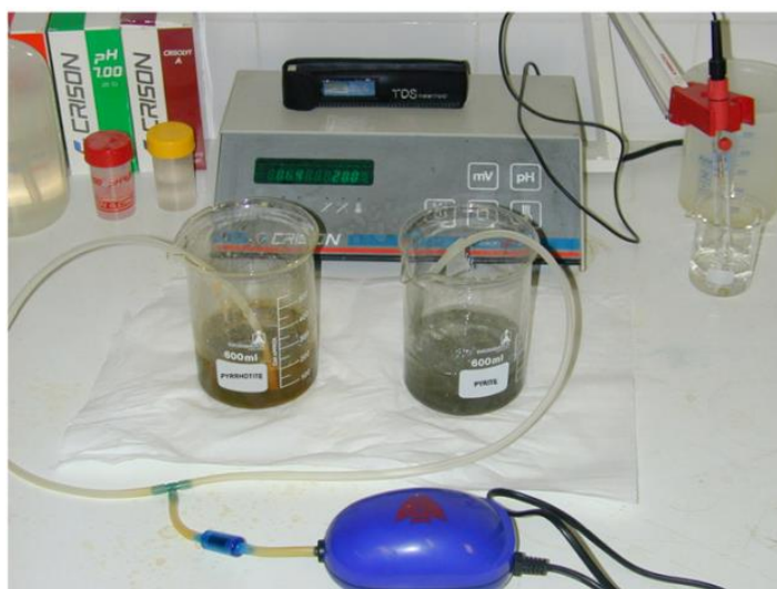
Figure 2.15: Oxygenation of pyrite and pyrrhotite samples (Chincón-Payá et al. , 2012)
