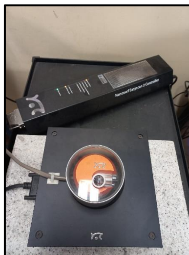
Figure 3.4.6. Nanosurf Scanning Tunneling Microscope, Easyscan 2. Photo taken in the Nanoscopia-UHV laboratory, at UFMG.
