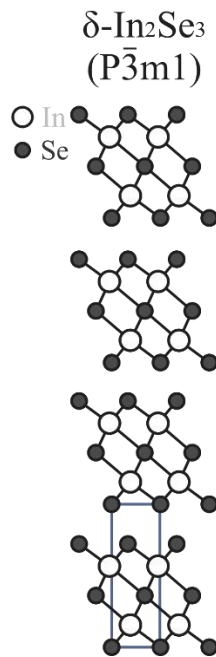
Figure 2.1.5. Schematic representation of the atomic structure of the \delta -In 2 Se 3 along the c -direction. The stacking of quintuple layers in the c -direction occurs without any rotation, translation, or reflection. Figure adapted from reference [38].
