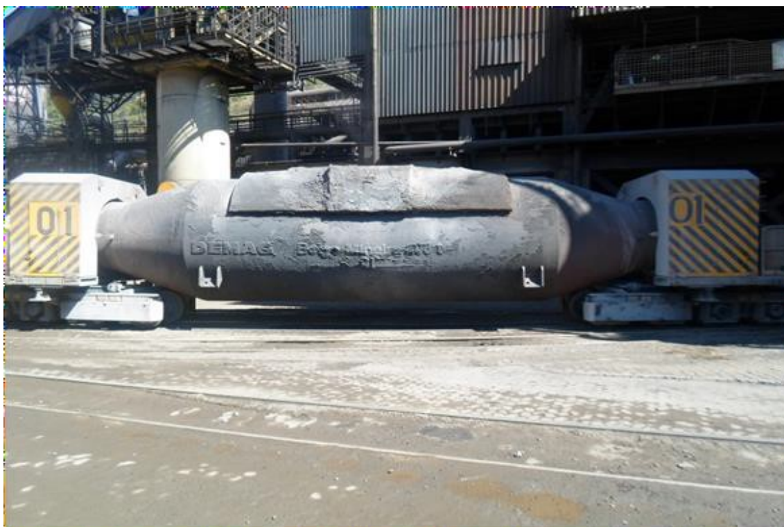
Figura 3.6. Carro Torpedo (Foto Interna – ArcelorMittal Monlevade)
