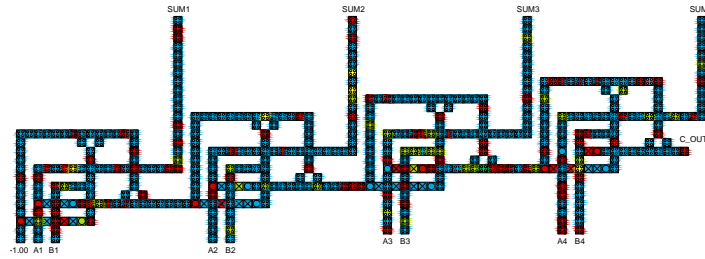
(a) RCA1 under combined defects.
