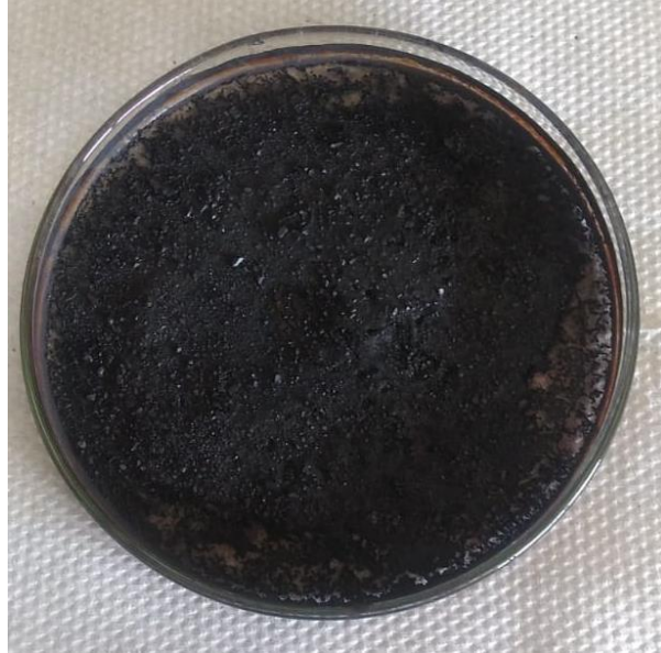
Figure 1: Magnetic adsorbent synthesized ( \text{Fe}_3\text{O}_4\text{-IL-Ni}^{2+} )
