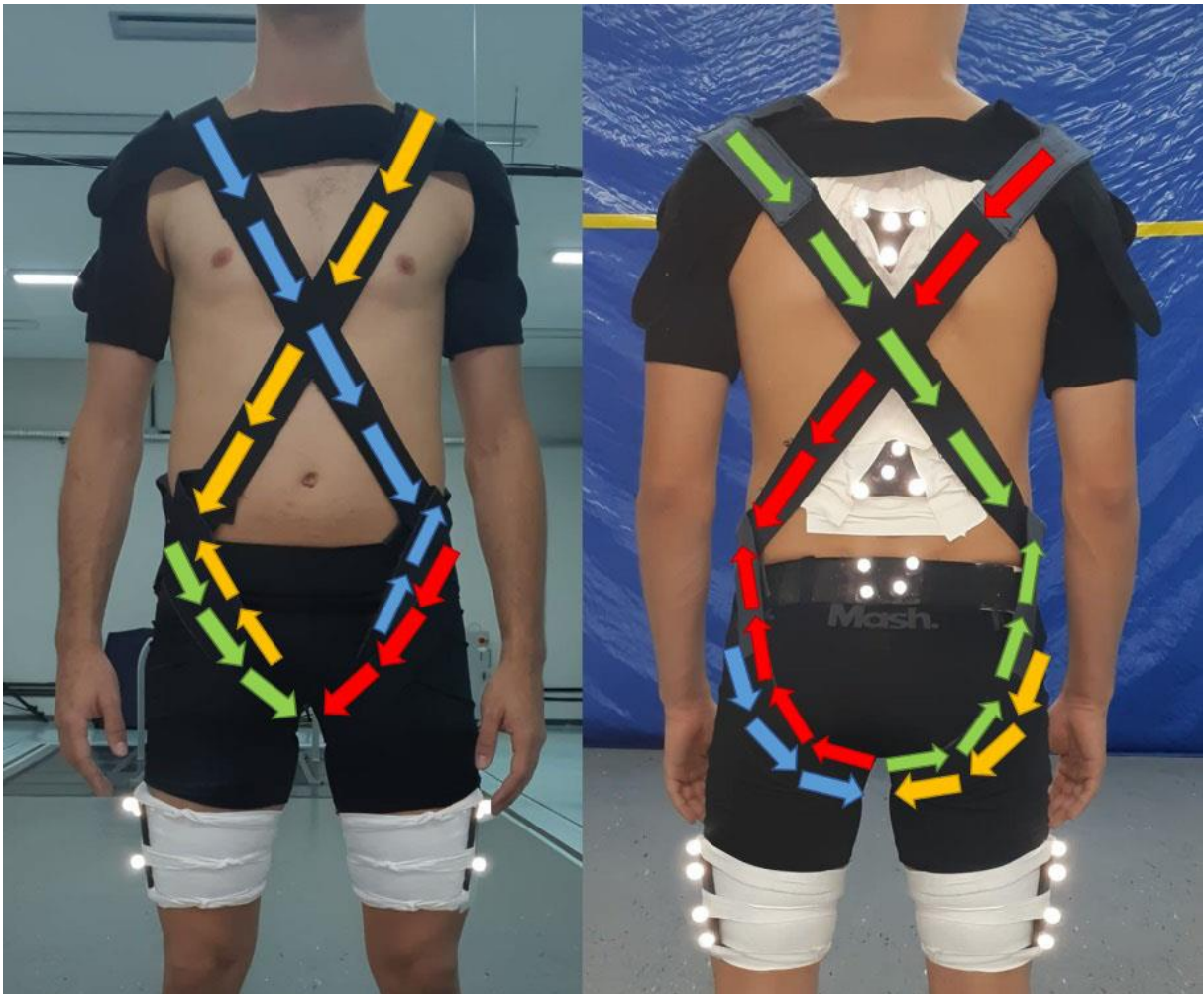
Figure 2. Image of the elastic bands fixed on the anchoring points - anterior and posterior views. Each of the four bands is represented by a different color (blue, green, yellow, and red) and the arrows indicate the direction of each band from proximal anchoring (shoulders) to distal anchoring (hips/groin).
