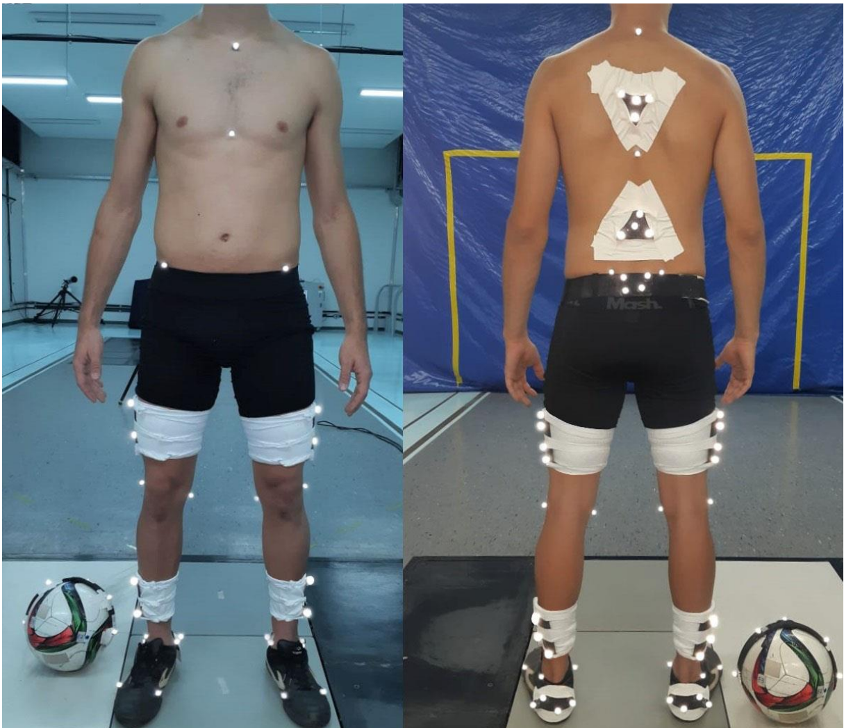
Figure 3. Photo indicating the clusters with clustered tracking markers used to track the movement of the segments: upper trunk, lower trunk, pelvis, thighs, legs and feet. The figure also shows the technical markers used for defining the segments' sizes and coordinate systems. They were placed on: jugular notch, T1 transverse process, xiphoid process, posterior projection of the xiphoid process, anterosuperior and posterosuperior iliac spines, medial and lateral epicondyles of the femur, medial and lateral malleoli, head of the first and fifth metatarsals.
