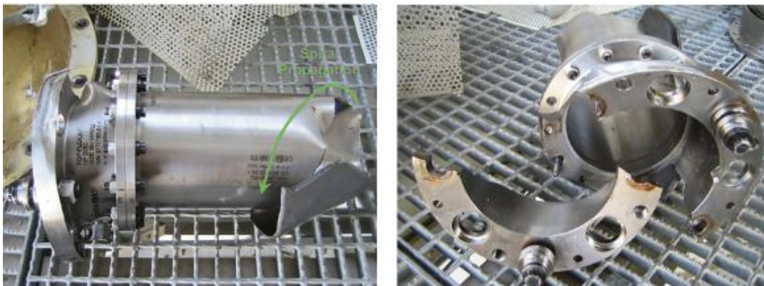
Figure 2: Disc coupling fatigue failure caused by torsional vibration in a VFD motor driven compressor train (Corcoran; Kocur; Mitsingas, 2010)
