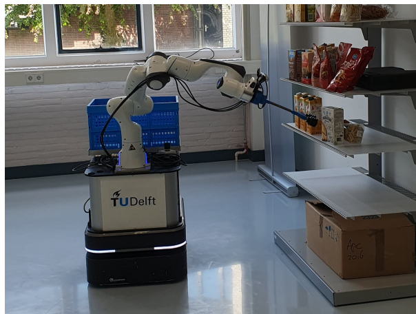
Figure 2.1: Mobile Manipulator performing a pick-and-place action using suction cups for supermarket applications, at TU-Delft during 2024 Robotics: Science and Systems conference. [90]
