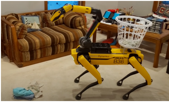
(a) Spot-arm [23]. A quadruped robot with a manipulator arm collecting clothing and placing it in a basket.
