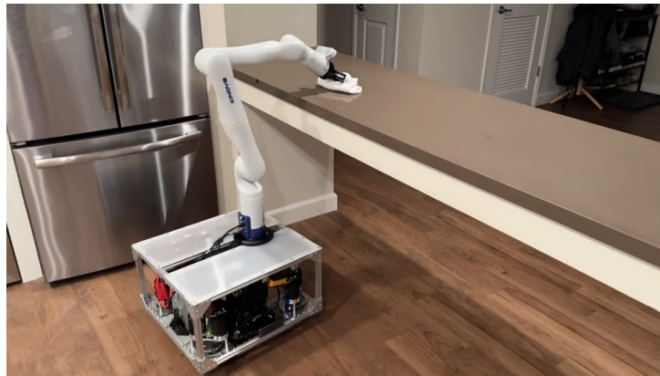
Figure 2.7: Mobile manipulator Tidybot++ cleaning a countertop [100].
