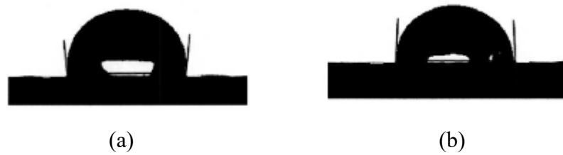
Fig. 3. 8 – Contact angle measurements of (a) new membrane and (b) 32,200 minutes irradiated membrane
