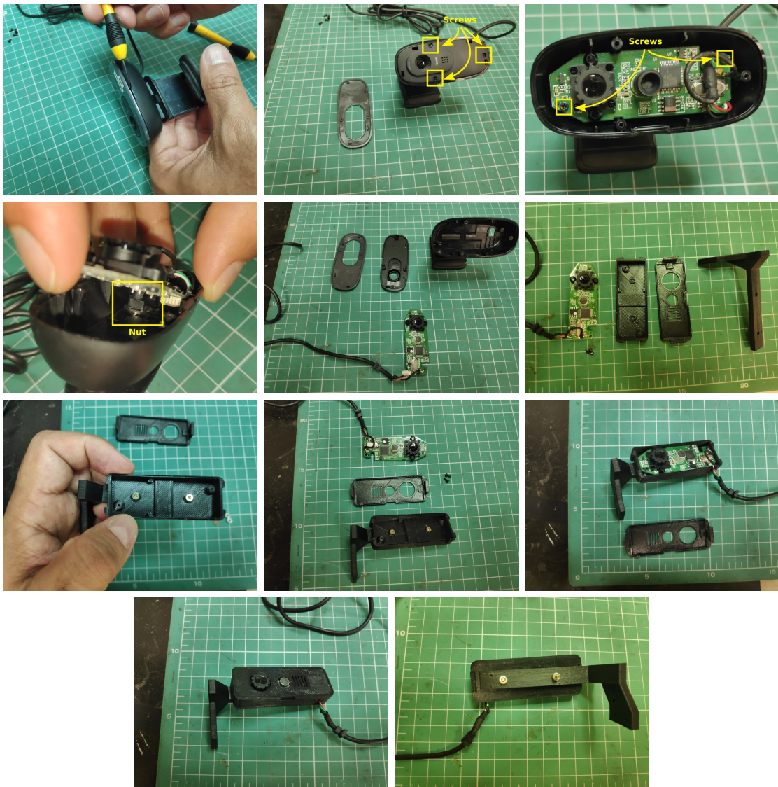
Figure A.6: C270 disassembly steps. (a) Frontal outer plastic removal. (b) Frontal case screws removal. (c) Circuit screws removal. (d) Nut holding circuit wire. (e) Original camera parts. (f) Camera circuit and printed case (g) World camera support and camera case (h) Final parts. (i) Camera circuit assembled on printed camera case. (j-k) Final result.
