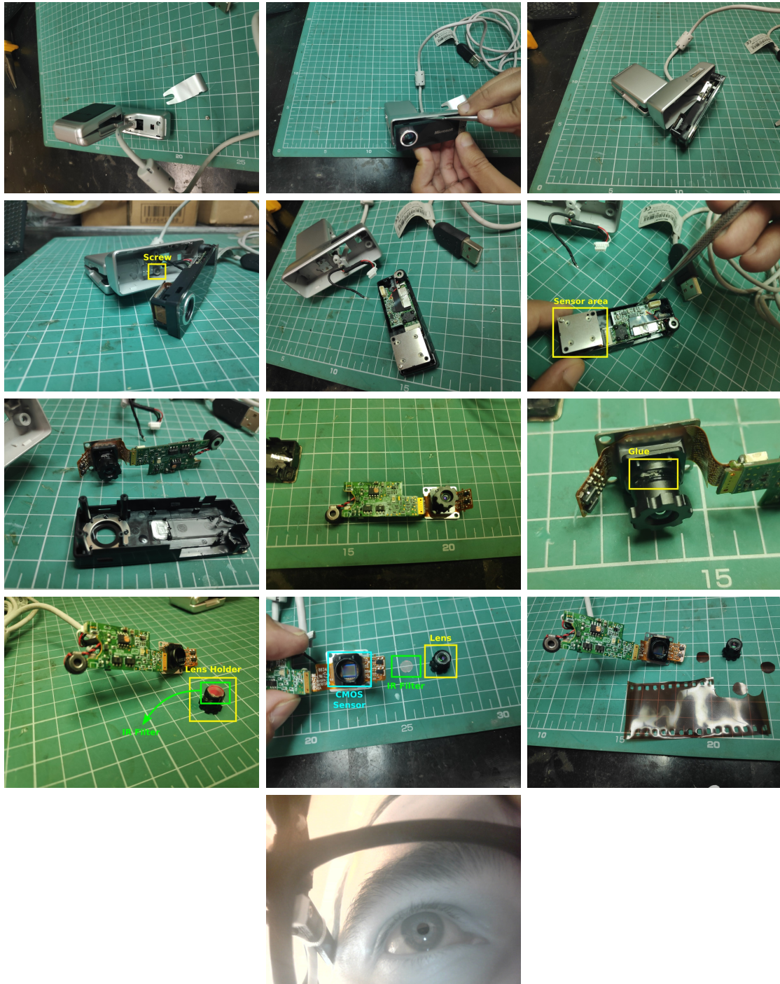
Figure A.7: VX-7000 disassembly steps. (a) Camera back screw removal. (b-c) Camera front removal using a tool. (d) USB wire removal. (e) Disconnection of USB cable. (f) Sensor area screws and detaching from front camera case. (g) Camera circuit and front camera part. (h) Camera circuit. (i) Lens holder on top of CMOS sensor. (j) Lens holder and camera circuit. (k) Top view from CMOS Sensor, IR Filter and Lens set. (l) Camera parts and cutted photographic film. (m) Image obtained from assembled camera, with IR-pass filter.
