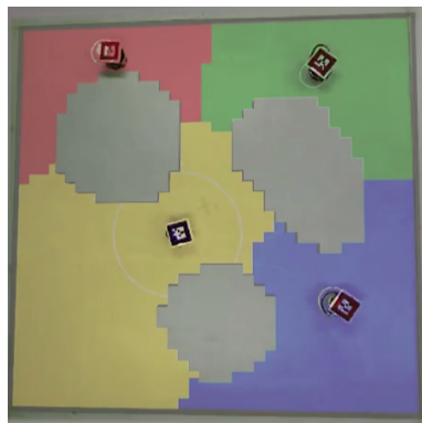
(e) Distribution of the robots around the Gaussian shaped density function placed around the center of the area, at t = 270s
