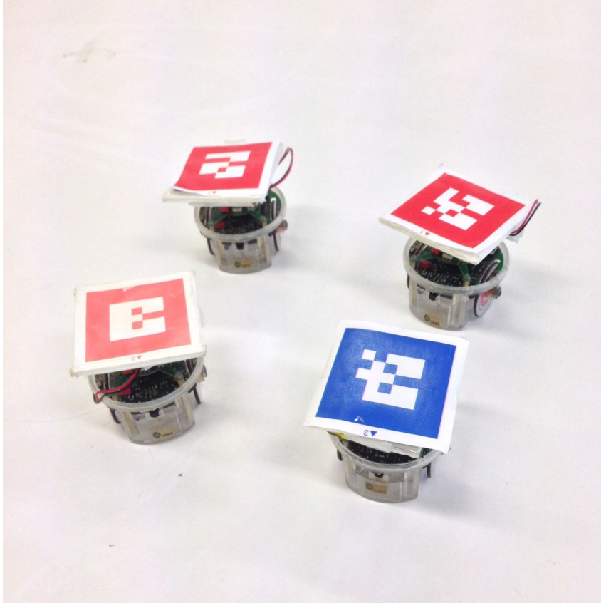
Figure 4.7: Team of e-puck robots used in the experiments.
