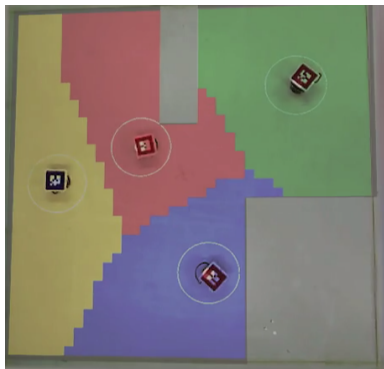
(e) Robots converge to a Gaussian shaped density distribution in the left side of the area at t = 255s .
