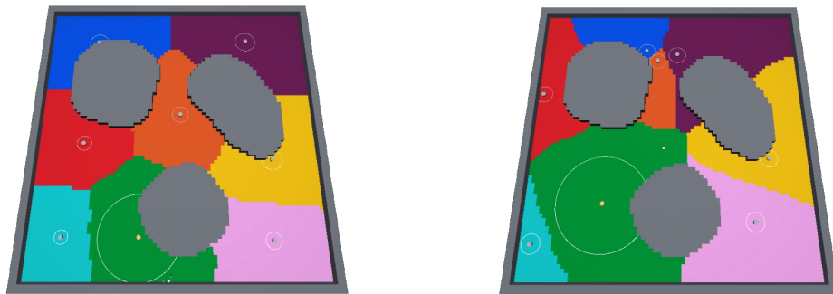
(c) Robot 1 with increased weight and a larger Voronoi region than in Figure 4.1b (d) Convergence showing robots attracted by a Gaussian density function.
