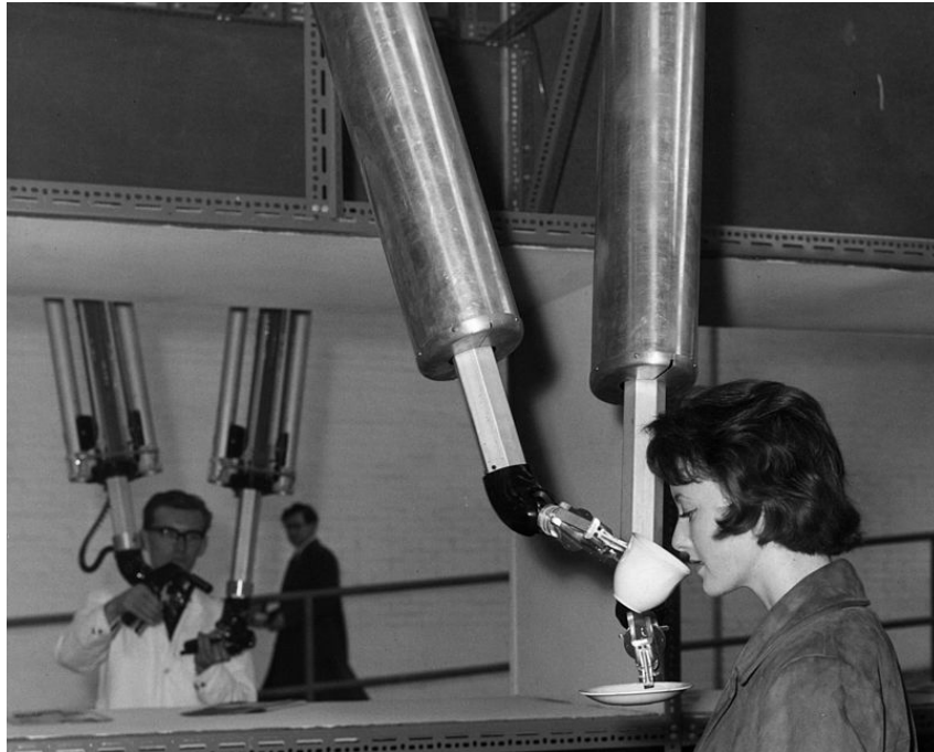
Figure 1.7: The Master Slave Manipulator Model NE9, developed for manipulation of nuclear material and one of the first human-robot interaction interfaces.
