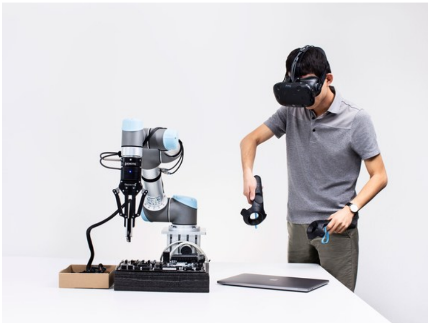
Figure 1.9: A human teleoperating a robot using a Virtual Reality headset.
