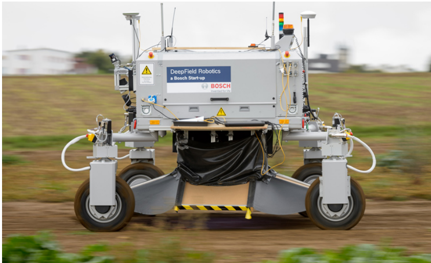
Figure 1.2: The BoniRob, a robot developed by Bosch for agriculture.
