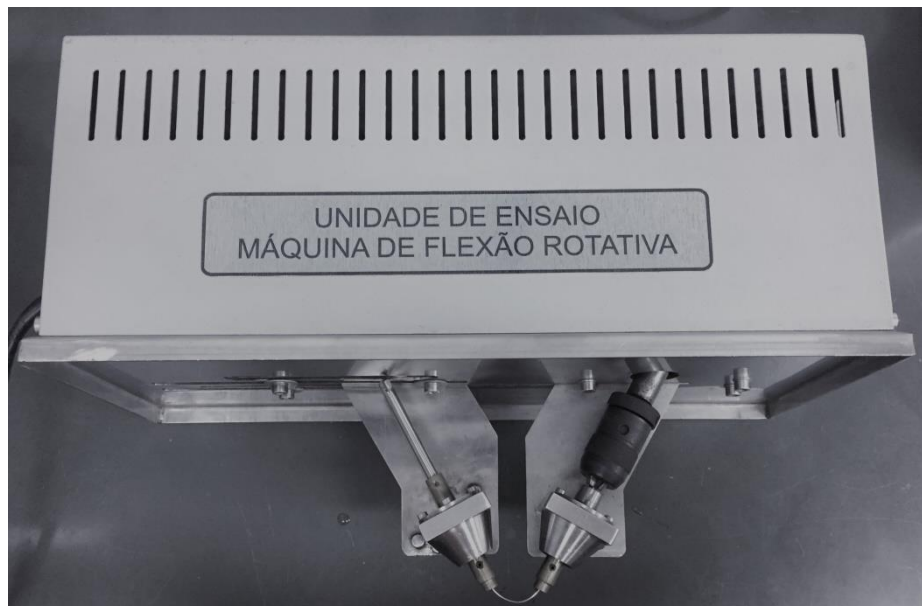
Figure 5.1 – Bending-rotating fatigue test apparatus.
