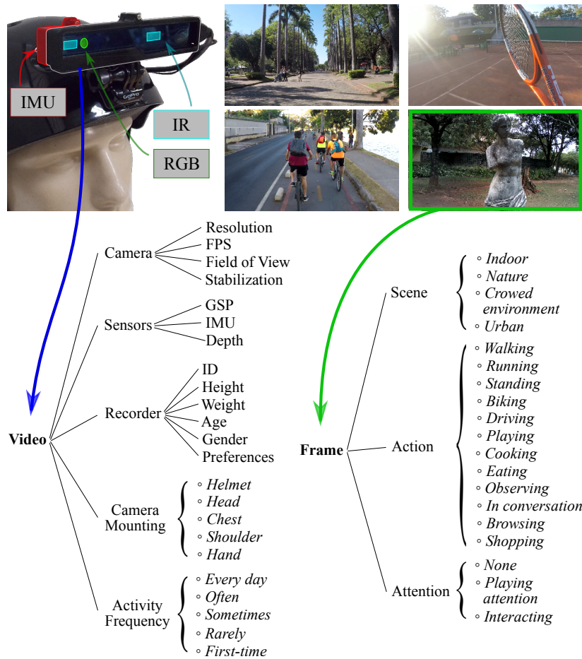
Figure 4.2. Sample and labels of the Dataset of Multimodal Semantic Egocentric Videos (DoMSEV). Top-left: setup used to record videos with RGB-D camera and IMU. Top-right: frame samples from DoMSEV. Bottom: Annotated information for videos and frames. The symbol \circ indicates the possible values for the respective annotation.
