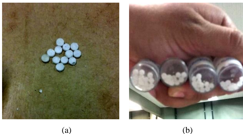
Figure 7.1 Chip-shaped samples of PMMA+HAp bone cement (1:1 ratio) and PMMA
