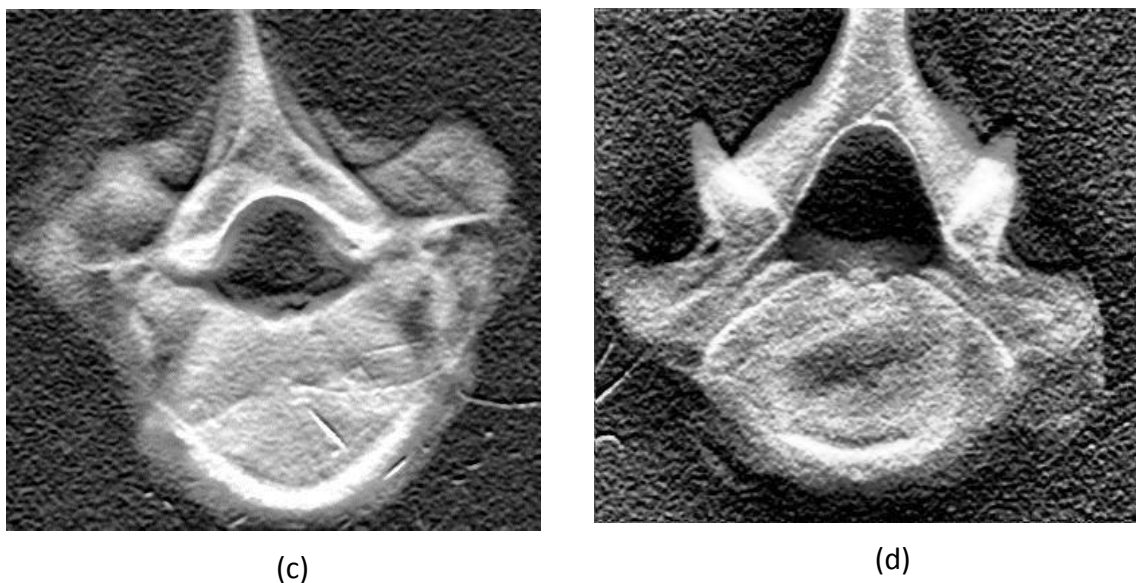
Figure 3.2 Radiological images of four vertebral models. In (a) the vertebrae have molten lead (b) PMMA injected. (c) PMMA + 10% BaSO 4 were injected. (d) x = 0.5 of the bone cement.
