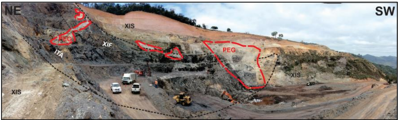
Figure 3.4: An overview of the Horto-Baratinha main pit, with the location of the units identified: XIS (mica-schist unit), XIF (amphibolitic schist unit), ITA (itabirite and iron ore), PEG (pegmatite). The dotted lines represent the contacts.
