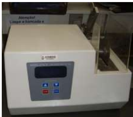
Figura 4.30 - Máquina de cortes Low Speed Precise Saw
