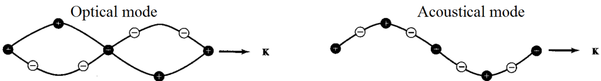
Figure 2.7 – Schematics of the optical and acoustic phonon modes in a diatomic linear lattice. Extracted from [27].
