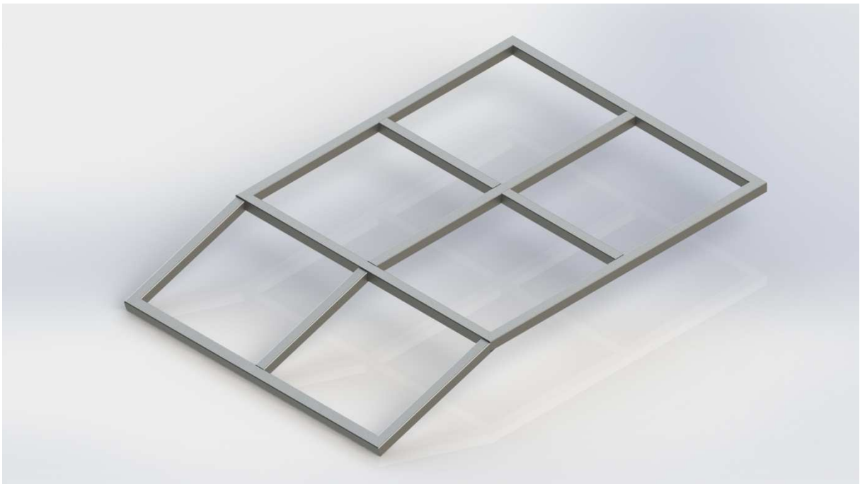
Figure 12 - Grid supporting the sheet metals Source: (COSTA e VICTORINO, 2019).
