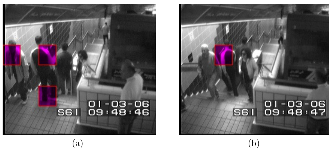
Figure 4.9: Examples of true positive matches for the exit gate clip.
