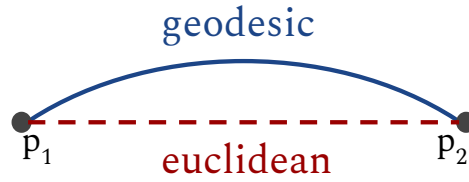
Figure 3.6: Geodesic (solid blue line) and euclidean distance (dashed red line)
