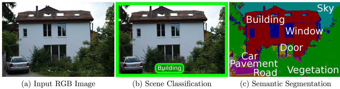
Figure 2.8: Example of an image processed by an scene classification and semantic segmentation algorithm Hazirbas [2014].
