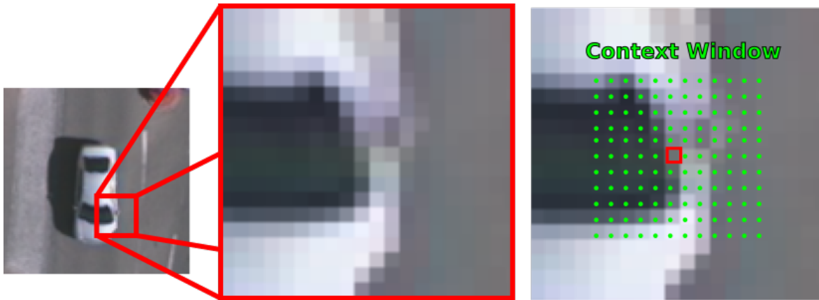
Figure 4.1: Representation of a context window, the green labels mark the pixels used for context and the red label notes the pixel being evaluated by the network.
