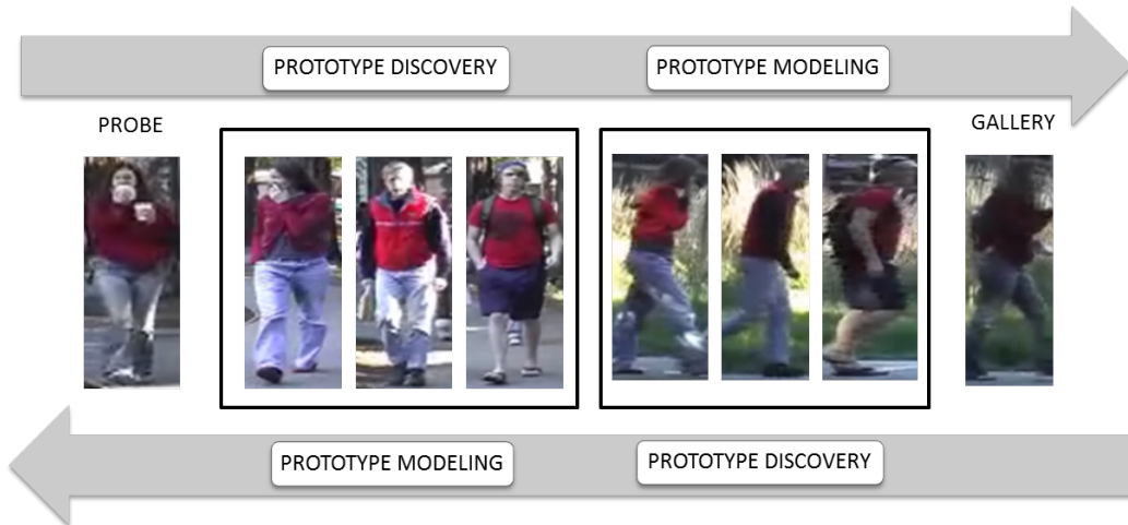
Figure 4.1: For a given sample (probe or gallery image), we compute the similarity with training samples captured by the same camera to determine the most similar individuals, which constitute the prototypes. Then, we use the class information to transit to the opposite camera where the models are learned and deployed.
