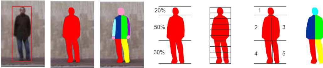
Figure 2.2: From left to right. First we have the pedestrian detection, foreground segmentation and the body segmentation. Then, different strategies of body segmentation are presented. The first two consider a fixed number of stripes, while in the last two we have five body parts obtained using human body symmetry [Farenzena et al., 2010]. Illustration taken from [Vezzani et al., 2013].
