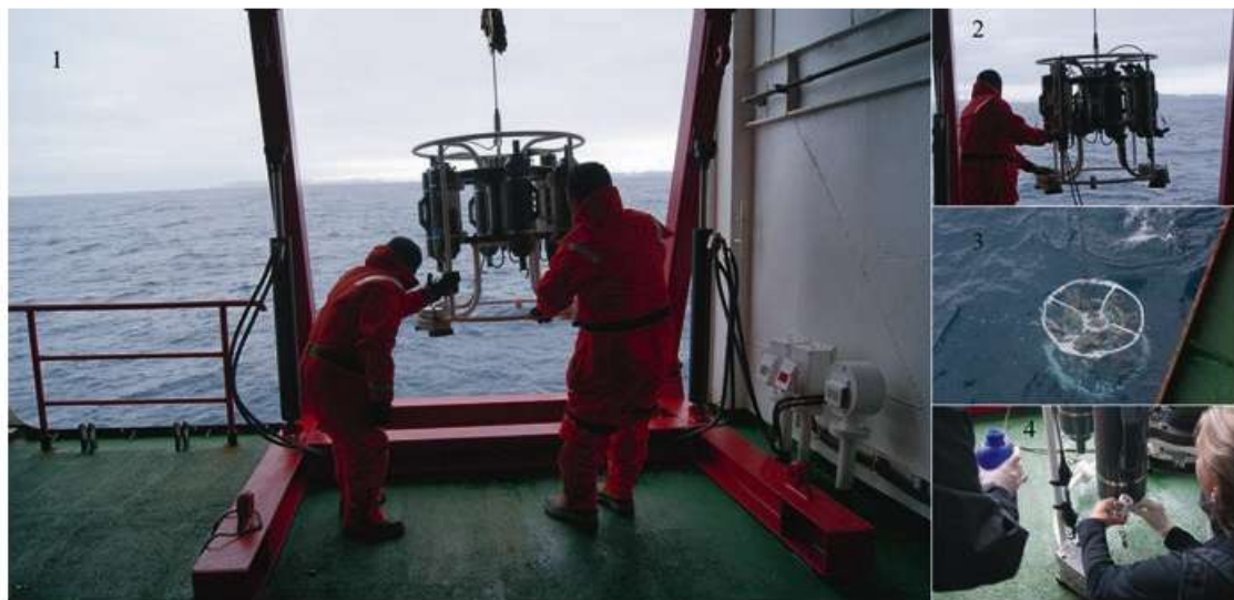
Fig. 10.7 Sequential process of seawater sampling using a combined Sea-Bird CTD equipped with 24 5L Niskin Sampling Bottles. (Photos Credits: LH Rosa)
