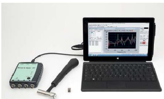
Figura 70 - Sistema USB 2.0-Powered Real-time Analyzer for Sound and Vibration Analysis Fonte: Manual Brüel & Kjær Sound & Vibration Measurement A/S
