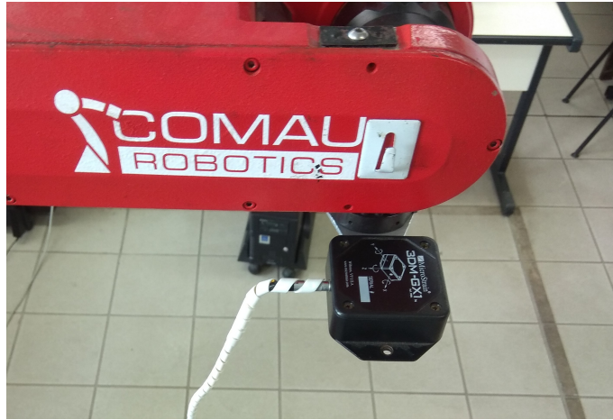
FIGURE 6.1: Experimental setup using the MicroStrain 3DM-GX1 ® IMU and the Comau Smart Six robot.
