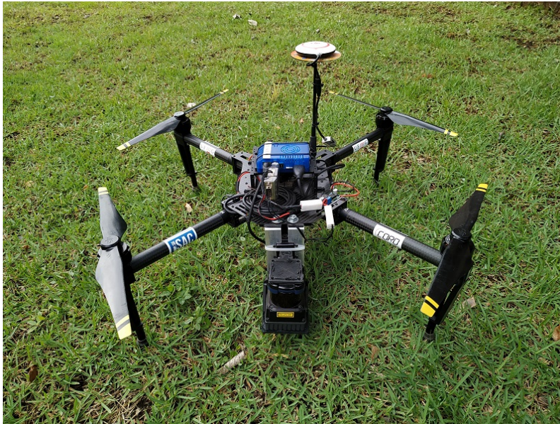
FIGURE 7.1: The quadrotor Matrice 100 DJI used in the state estimation experiment. The vehicle is commercialized with built-in AHRS and GNSS, and was equipped with a Hokuyo UTM-30LX-EW planar LiDAR.
