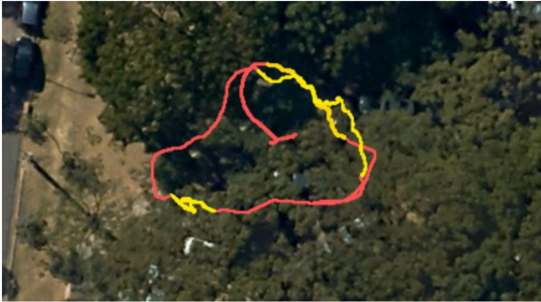
FIGURE 7.14: Satellite view of the forest where our onboard experiments were executed. Image provided by Google Maps. The path estimated by RAUKF-CM \chi^2 is shown in red, when AHRS, LO, and GNSS were available and in yellow GNSS was unavailable.
