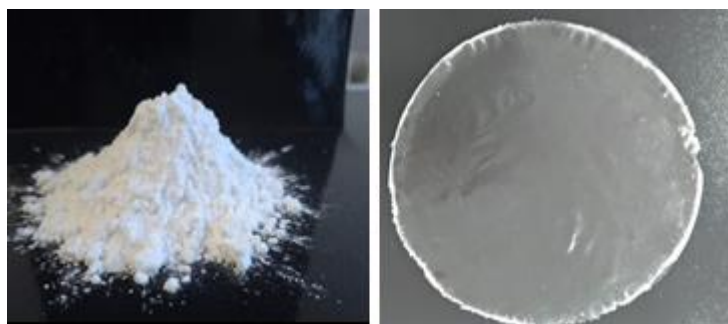
Fig. 1 – Commercial Corn Starch powder (left) and the resulting bioplastic film after casting (right).
