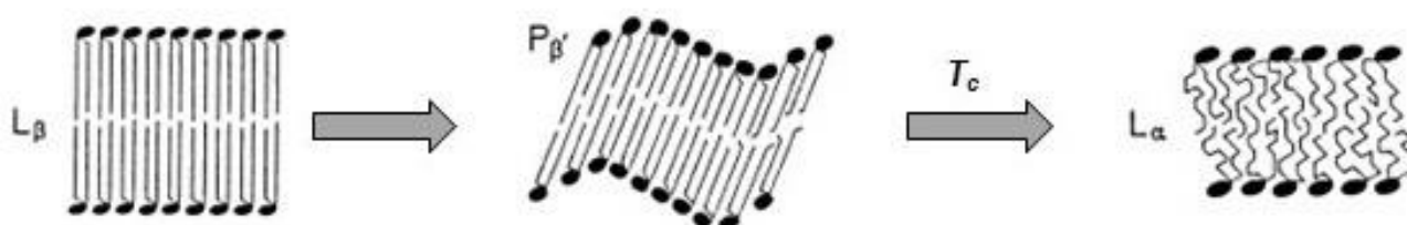
Figure 8 – Schematic representation of L\beta \rightarrow L\alpha phase transition.
