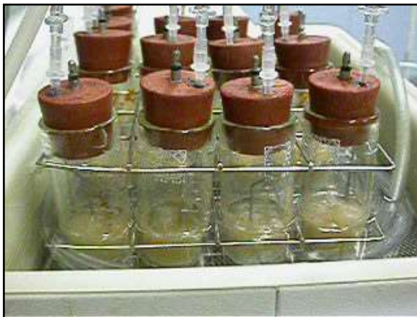
Figure 3.3: Photo of the physiologically based extraction test (PBET) apparatus containing the required enzyme
