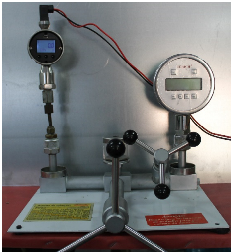
Figure B.1: Pressure calibrator used for verification.
