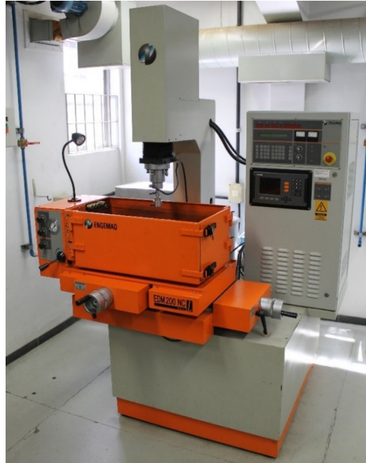
Figure 3.3: EDM machine used to cut the capillary tubes.
