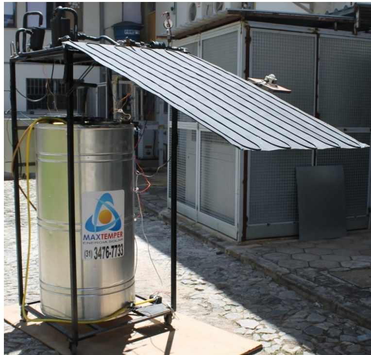
Figure 3.9: Overview of the CO 2 DX-SAHP.
