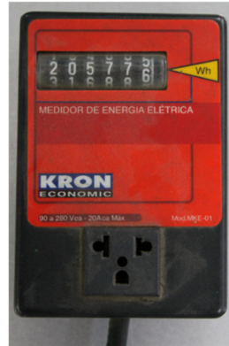
Figure B.4: Electrical energy meter.
