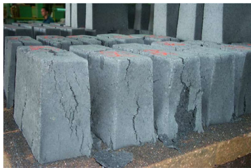
Figure 5 - Hydration of doloma bricks during process manufacturing (Source: RHI Magnesita).
