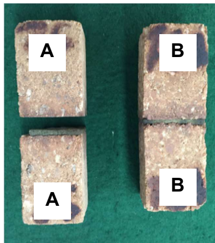
Figure 39 – Visual aspect of bricks A and B after the sandwich coating test modified in the present work.
