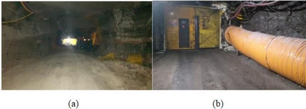
Figure 7- (a) without air regulator; (b) application of regulator and doors for air redistribution
