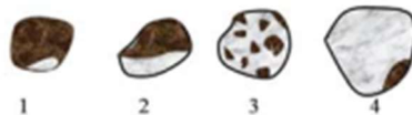
Figure 2.3. Different products of comminution exhibiting different liberation patterns Source: WILLS and FINCH, 2016.
