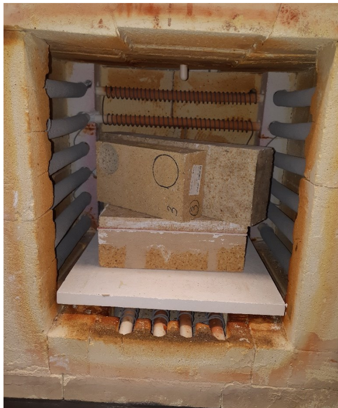
Figure 4.3: Closed box containing the sample bricks and positioned inside a furnace.
