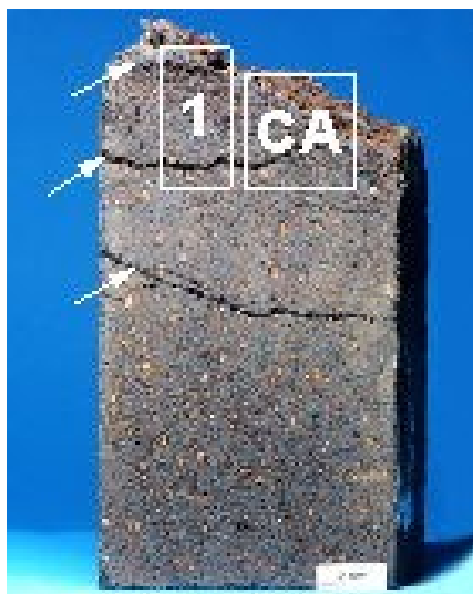
Figure 1.2: Brick taken from a nickel flash smelting furnace, showing cracks parallel to its hot face (arrows). Sections were cut from the hot face for microscopic (1) and chemical (CA) examinations.
