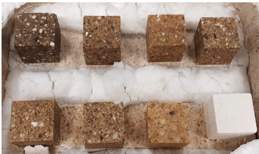
Figure 5.3: Visual aspect of the refractory samples after corrosion test I
