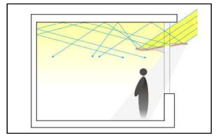
Figure 2. Scheme of the natural light reflection in the built space from the installation of the light shelf
