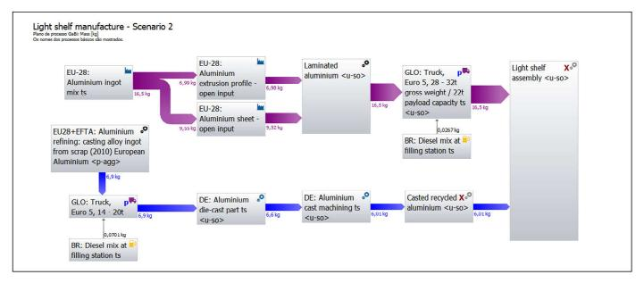
Figure 4. Life cycle inventory of the Light shelf - Scenario 2 (side parts from recycled aluminum)
