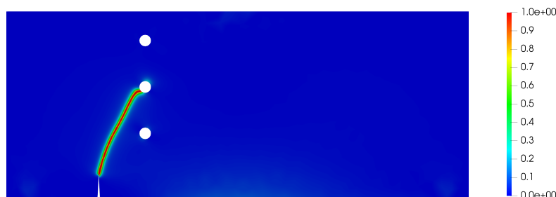
Figure 9.12: Phase-field profile for asymmetrically notched beam in 120th step.
