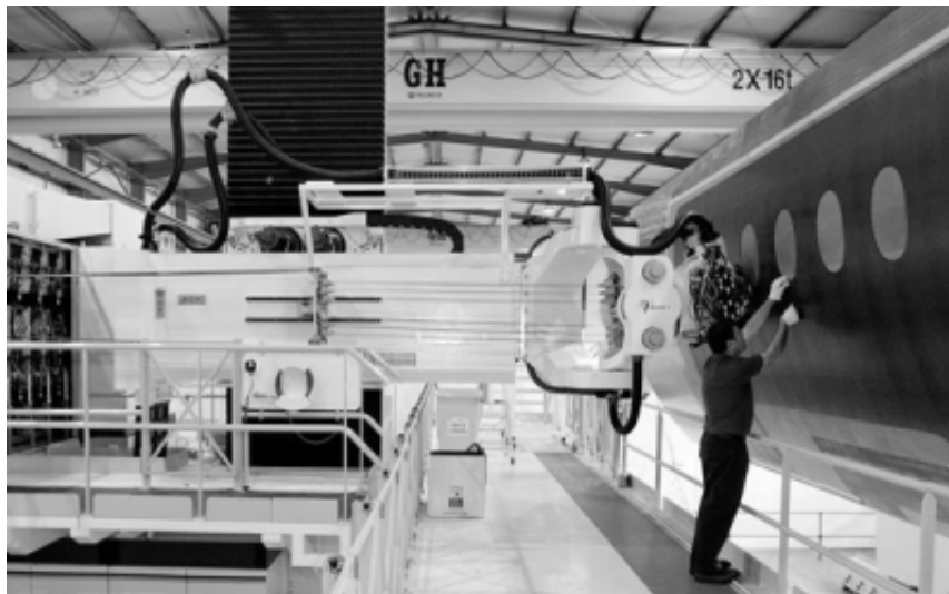
Figure 1.5: Fiber placement machine laying on a fuselage section (source: Mtorres).
