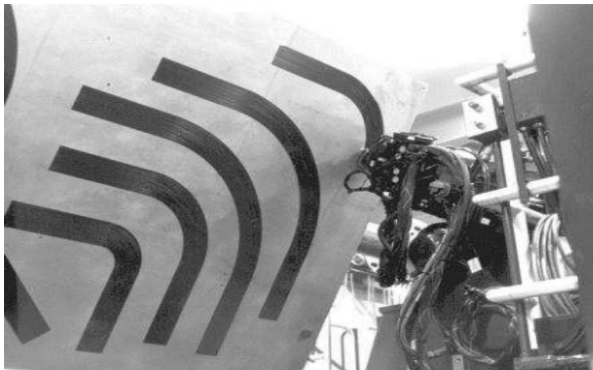
Figure 1.6: Steered fibers disposed by a AFP machine (source: Ingersoll Machine Tools).
