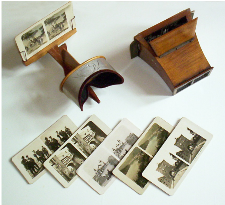
Figure 6 - Holmes stereoscope (left), Brewster stereoscope (right) and some cards with stereoscopic images. The latter provides a more intimate experience. Albers, Dieter. “Stereoscope viewer, on display at Schulhistorische Sammlung”. 2009. Wikimedia. : https://bit.ly/3posnJe . Accessed 05 Feb. 2020.
