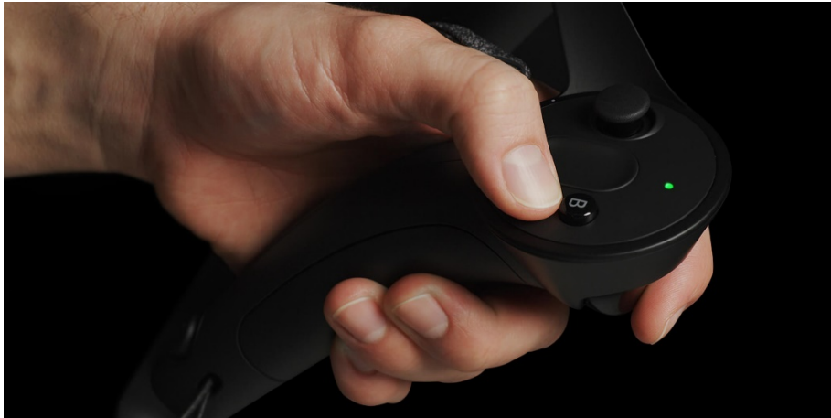
Figure 32 – The Valve Index Controller: 87 sensors to detect movements of the hand, fingers, and pressure. Valve. 2019. Retrieved from https://bit.ly/3j3qXBk . Accessed in 27 Jul. 2021.
