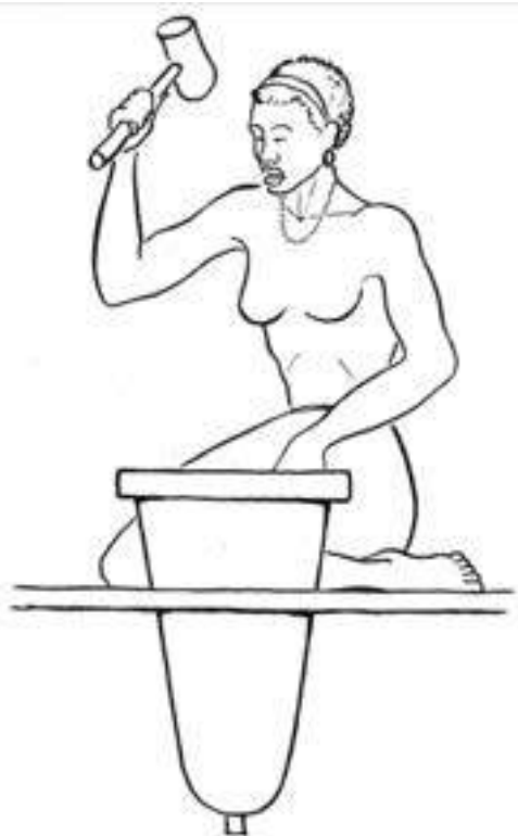
Figura 26 – Entaipar as fôrmas
