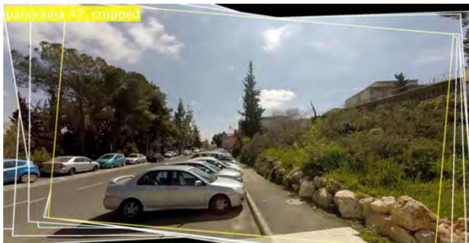
Figure 2.3. An output frame produced by the Halperin et al. [2018] method. They look into different directions and collect frames from the input video, creating mosaics around each frame. The mosaics are sampled to meet playback speed and video stabilization requirements. The different original frames are marked with white lines (extracted from Halperin et al. [2018])
