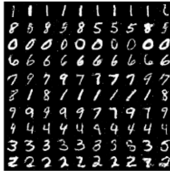
Figure 2.5. Example of result after training an architecture of 10 generators with the MNIST dataset, with each line corresponding to generated samples of one of the generators.
