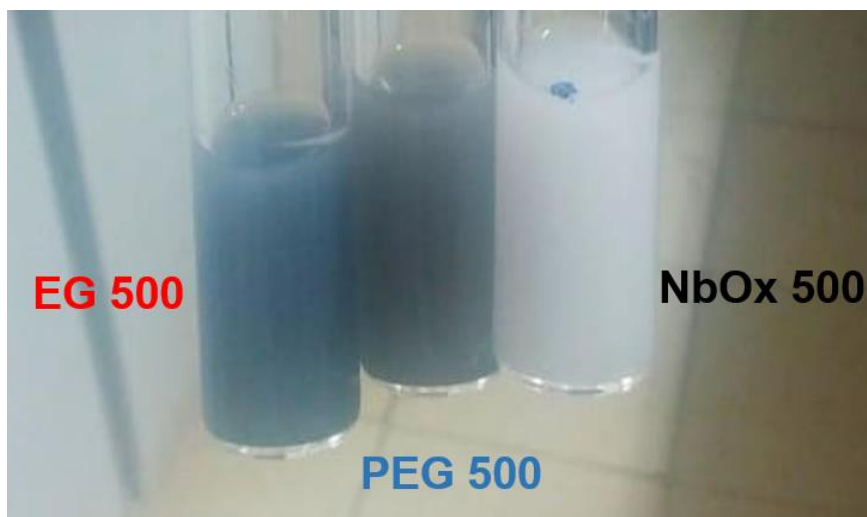
Figure 7. 8. Coloration changes during the electron accumulation phenomenon.
