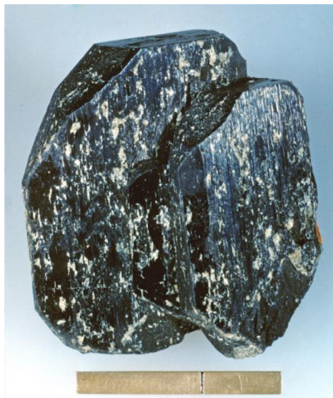
Figure 1. 1. Columbite ore - Evidencing the black color and the gold streaks – Image obtained from [3].
