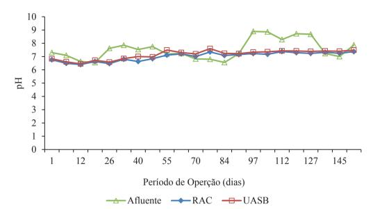
Figure 2. Influent and effluent pH values for the ABR and UASB reactors during the experimental period.
