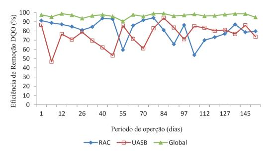
The ABR-UASB reactor system had an average removal efficiency of 96.7% for COD, with minor variations, showing high reliability and operational stability.
