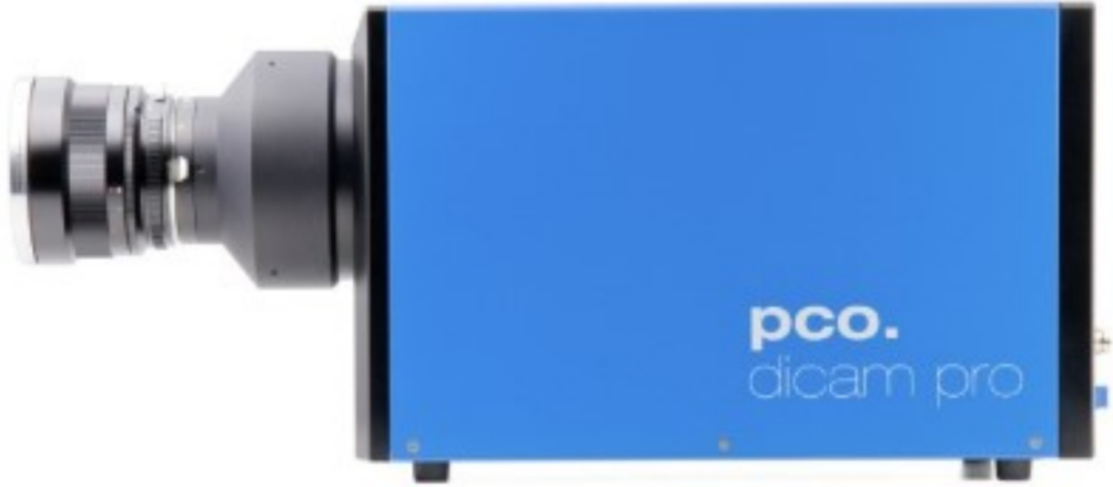
Figura 22 – Image of the intensified charged-coupled device (ICCD) camera used to perform the measurements at the experimental setup, Figure 15.
