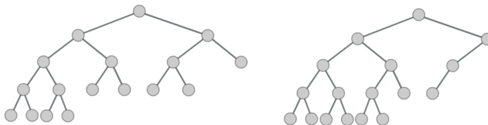
Fig. 3.1: Two searching trees with 17 nodes and minimal depth of 5, none of which correspond to binary searching.
