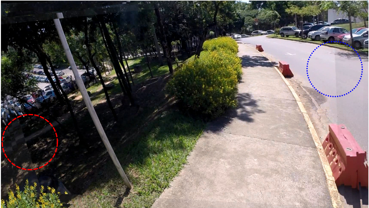
Figure 4.8. Planes mismatches, failure case 1. The Figure depicts a frame reconstructed by the stitching process. The usage of homography restricts the correct matches for only one plane per image. The blue dotted circle presents a region where the planes match correctly. The red dotted circle presents a region where the planes do not match correctly.
