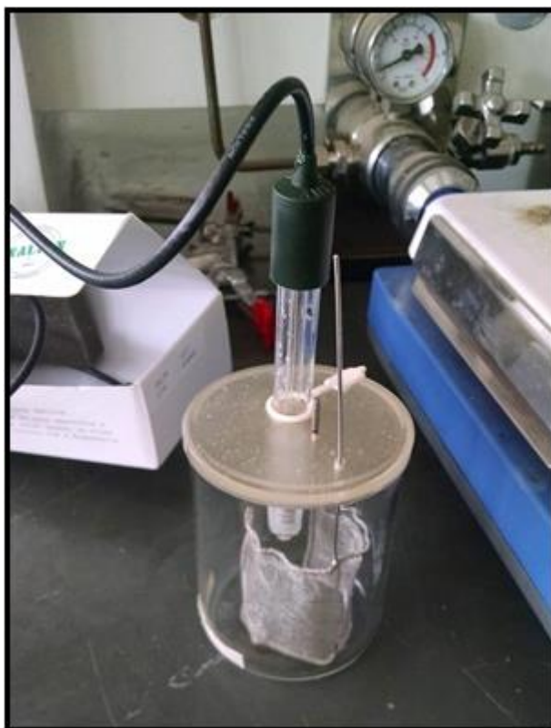
Figure 4.16 – Electrochemical cell used for CPP experiments
