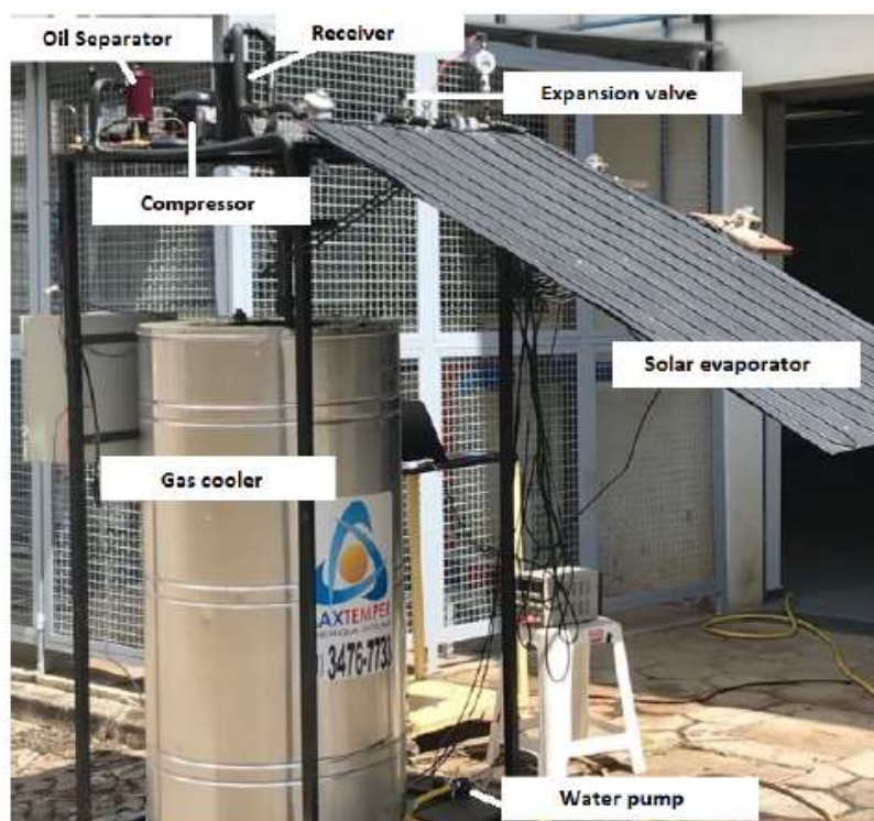
FIGURE 14 - Experimental device of CO 2 DX-SAHP.
