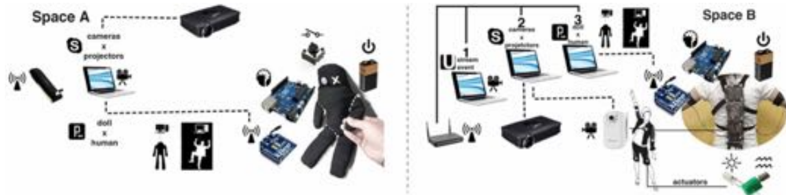
Figure 2. Sensor to actuator transmission and image exchange between spaces A and B (Copyright 2011, LAGEAR. Used with permission)
