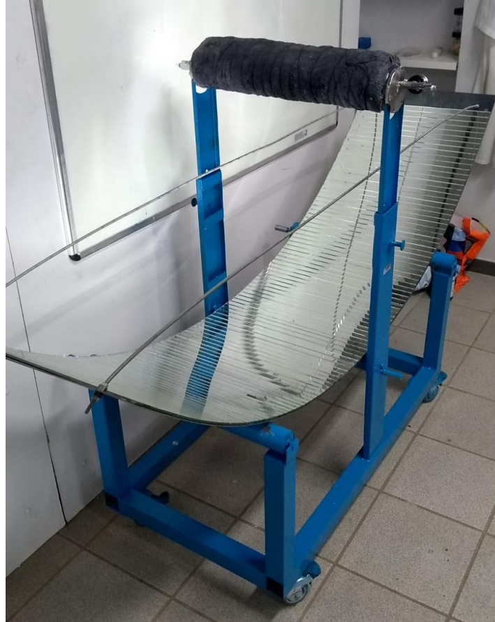
Figure 28 - Assembled parabolic trough solar pyrolyzer.
