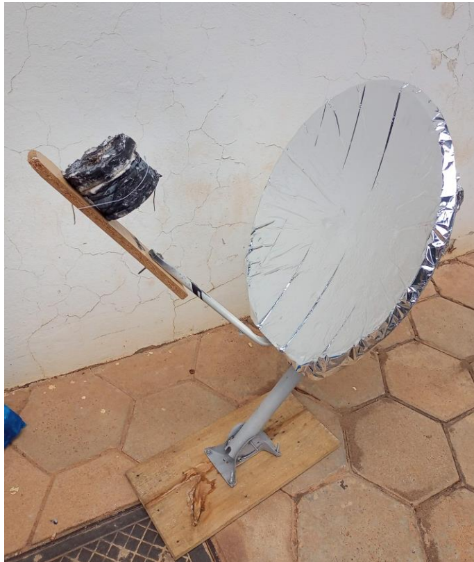
Figure 29 - Assembled parabolic dish solar pyrolyzer.
